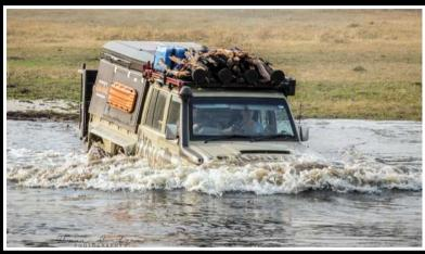
systems to gain up to 4 inches of lift. The design also allows for 6 snow tracks to be fitted if required. With the added weight, the brakes have received attention too. Discs are upgraded to 350 mm rotors with 6 pot callipers all round. The handbrake is mounted to the transfer case and locks the driveshafts
